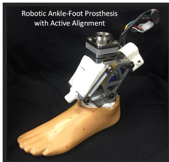
Fig. 1. Active alignment is a design feature that realigns the limb towards the center of pressure during stance phase of walking. Active alignment reduces peak moment transfer to the limb, resulting in reduced intra-socket peak pressures.
